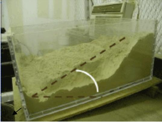
A continuous flow air supply was applied to the Demonstration Box containing Class C Fly Ash at a vertical velocity of 5ft/min. The continuous flow successfully discharged much of the Fly Ash, but could not remove the material below the 16 degree working angle (normal for Class C Fly Ash). PMT with multiple frequencies was then applied to the discharge air slide in front and the air-slide furthest to the left using only 3ft/min of air flow.
