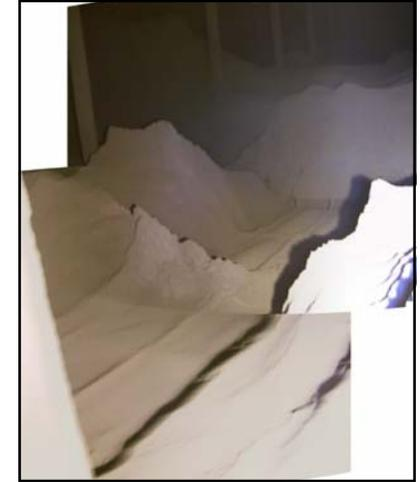
Above photo shows the result of trial, demonstrating the effect of Pneumatic Modulation Technology applied to just a few airslide panels.
